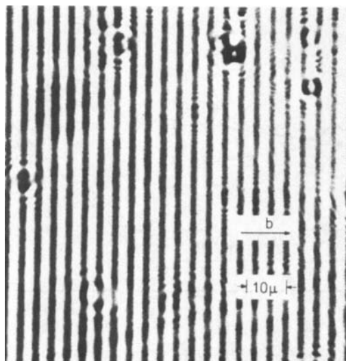
FIGURE 7. Photography of a holographic grating on a TS-crystal surface, taken in a light transmission microscope 6
